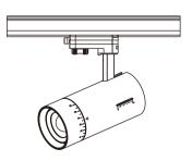
Adjust the illumination angle of the luminaire
